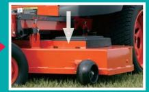
Push and release the pedal again to lower the deck
